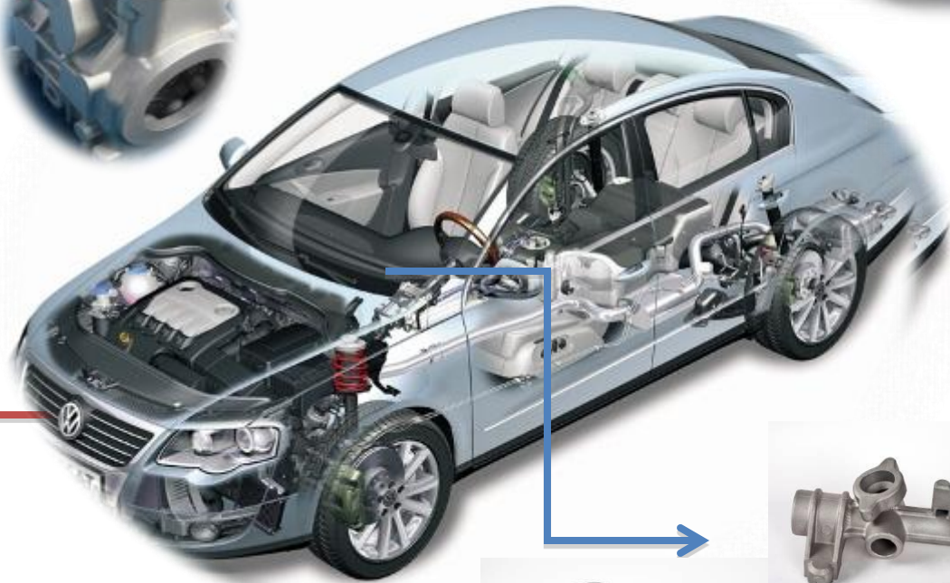
Part Name: Transmission Housing Material: AC3AM
