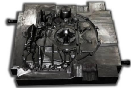
Part Name: Mold for Flywheel Housing Customer: Iveco
